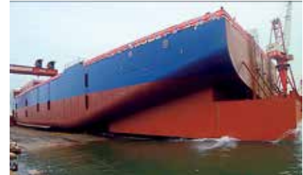
Launching of the hull from a slipway
